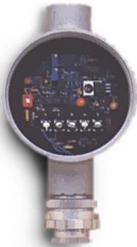
The RW720 Modulated carrier amplifier and analog transmitter is a meter mounted device designed to combine the advantages of the modulated carrier principle with the convenience of an analog output in a single assembly. It is a 2-wire Loop Powered Output system with RF
