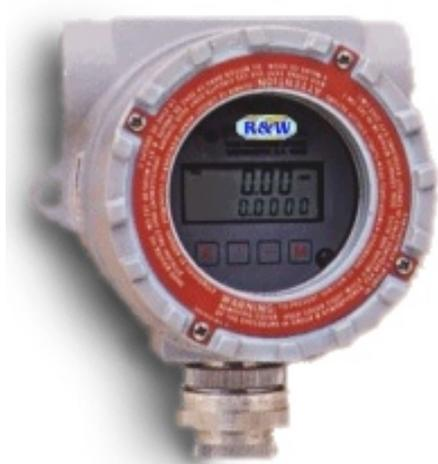
Model IT300N industrial remote totalizer/rate indicator is a battery powered device that provides flow totalization and rate indication in most engineering units. Additionally, 10-point linearization is available to enhance accuracy and extend a flowmeter's linear flow range. Rate and total are displayed by a 4-digit and an 8-digit liquid crystal display respectively. Alternate power can be provided by an external DC power supply or by a current loop.
