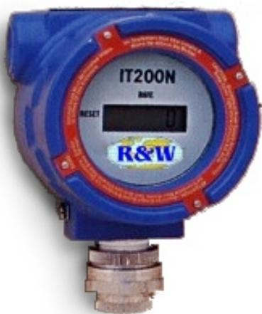
The model IT200N industrial remote rate indicator is a battery-powered device that provides flow rate in most engineering units. Rate is displayed via an eight digit Liquid crystal display. Selection of the reset function is accomplished
