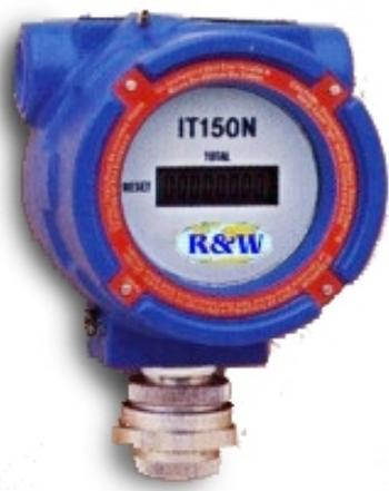
The Model IT150 industrial remote totalizer is a battery-powered device that provides flow totalization in most engineering units. Total is displayed via an 8-digit liquid crystal display. Reset of the totalizer is accomplished externally by a magnetic field. This
