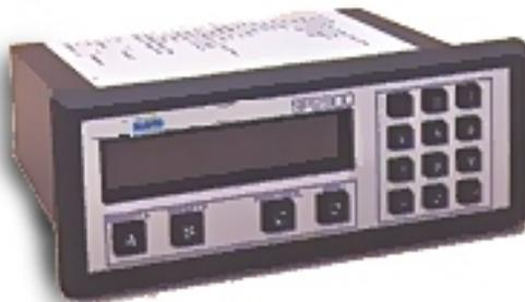
The model RW2850-TC is a Temperature or Density compensated batch Totalizer/Rate Indicator with selectable 16 pt. linearization. This unit allows viewing of batch total and flow rate indication. The RW2850TC features 8 digits of bright .55", alphanumeric display, and can accept up to 10KHz and a direct 100 Ohm platinum RTD or analog input. An 8-digit floating decimal, "K" factor convert, inputs to meaningful count and rate data. The user can easily view preset value, temperature,
