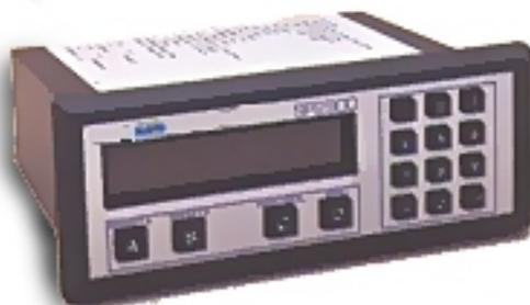
Model RW2800 combines three unique products into one easy-to-use field programmable device: batching, totalization, and flow rate. The batching counter counts to prewarn and preset numbers entered by the user and provides Separate control outputs. The totalizing counter provides accumulative or grand totals. The rate meter counts the
