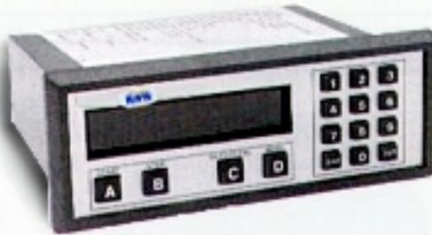
The RW2700 is a multifunction net flow Totalizer/Rate Indicator that measures flow in and out of a system. The RW2700 accepts two pulse inputs: subtracts B input from A and displays the net total flow A-B or net Rate A-B. Separate "K" factors can be entered via the front panel for
